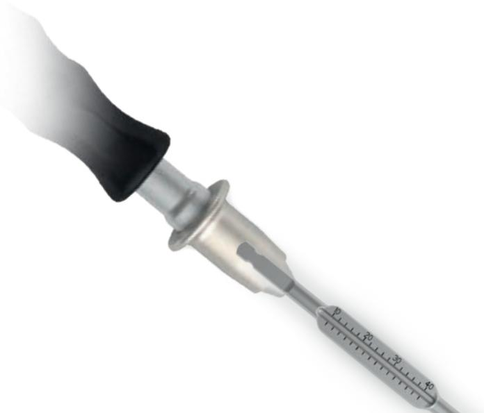
Use the counterink with depth gauge to prepare the first cortex and determine the length of the screw to be implanted: insert the counterink on the portion of the wire protruding from the bone and, in rotation, penetrate the first cortex as far as the instrument allows. In this position the back end of the wire (or the reference notch) will indicate, on the graduated plane of the instrument, the length of the screw to be implanted.
